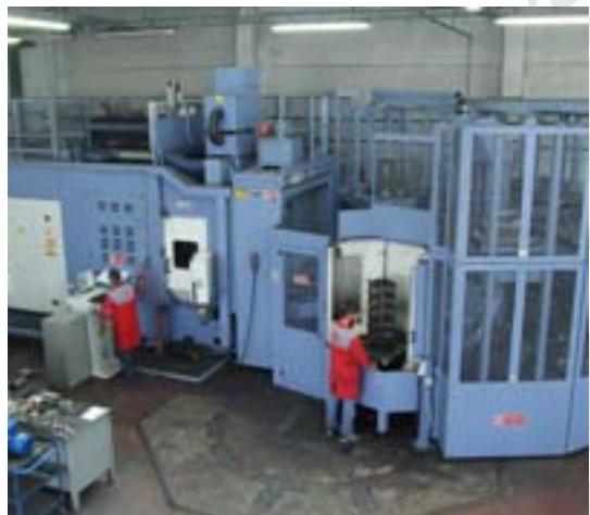
Numerically controlled machining center with 18 pallets.
