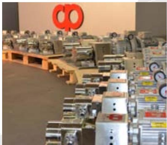
Gear metering pumps "N" for food plant.
